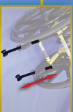
Rear anti tippers can be adjusted up or down
